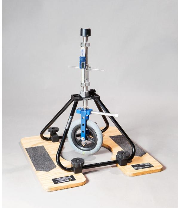
**Photo 8.26 - Rotational Penetrometer**
