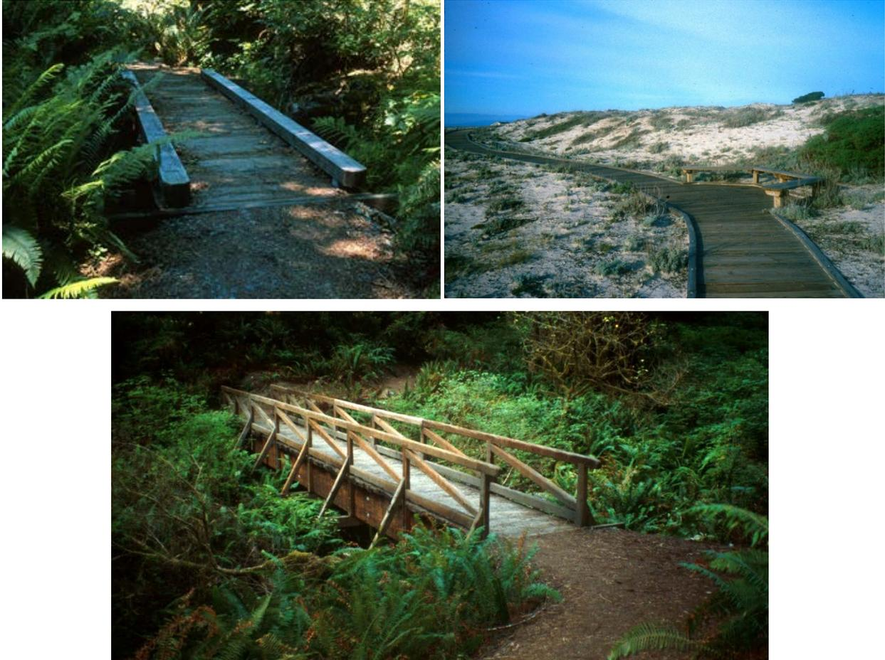
**Photo 8.24 - Puncheon (top left), Boardwalk (top right), and Bridge (bottom)**
