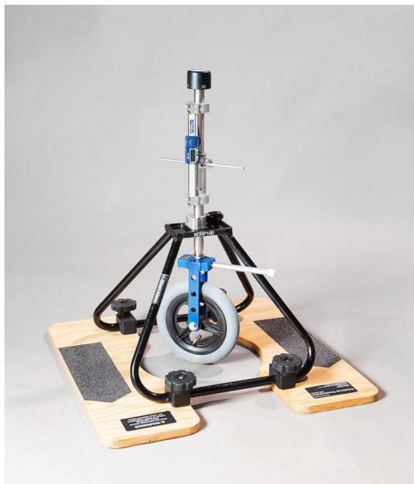
**Photo 8.26 - Rotational Penetrometer**
