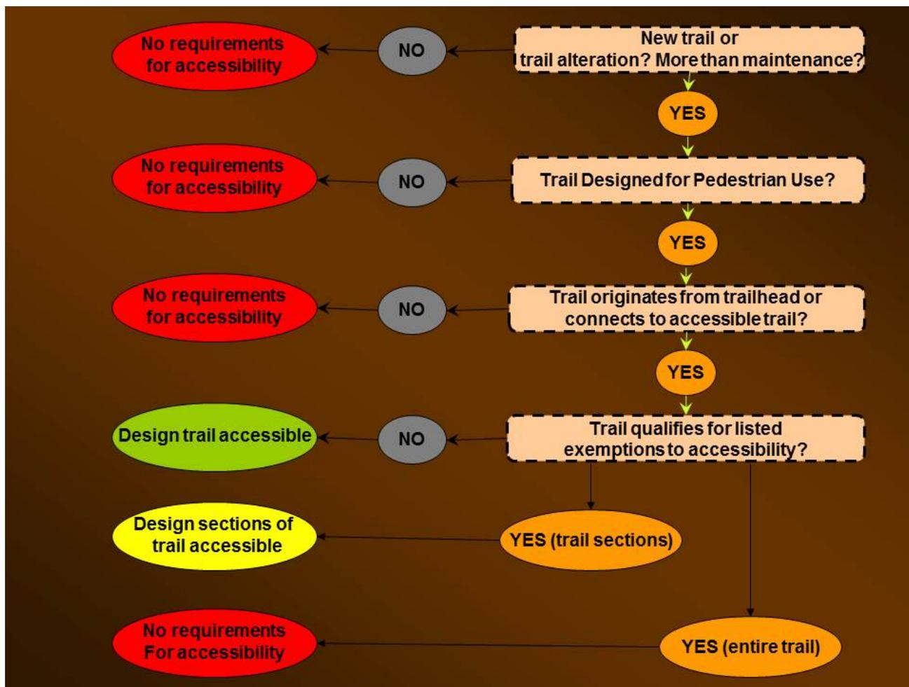
**Figure 8.1 - Accessibility Compliance Determination Flow Chart**
